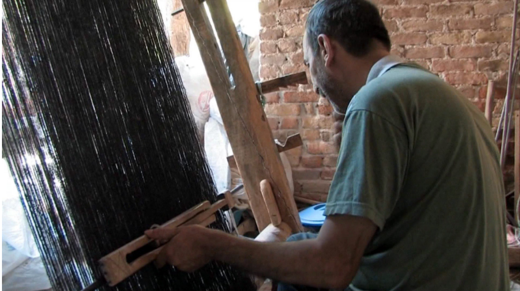
image 4.087: The weaver measures the width of the warp according to the desired design of the panel.
