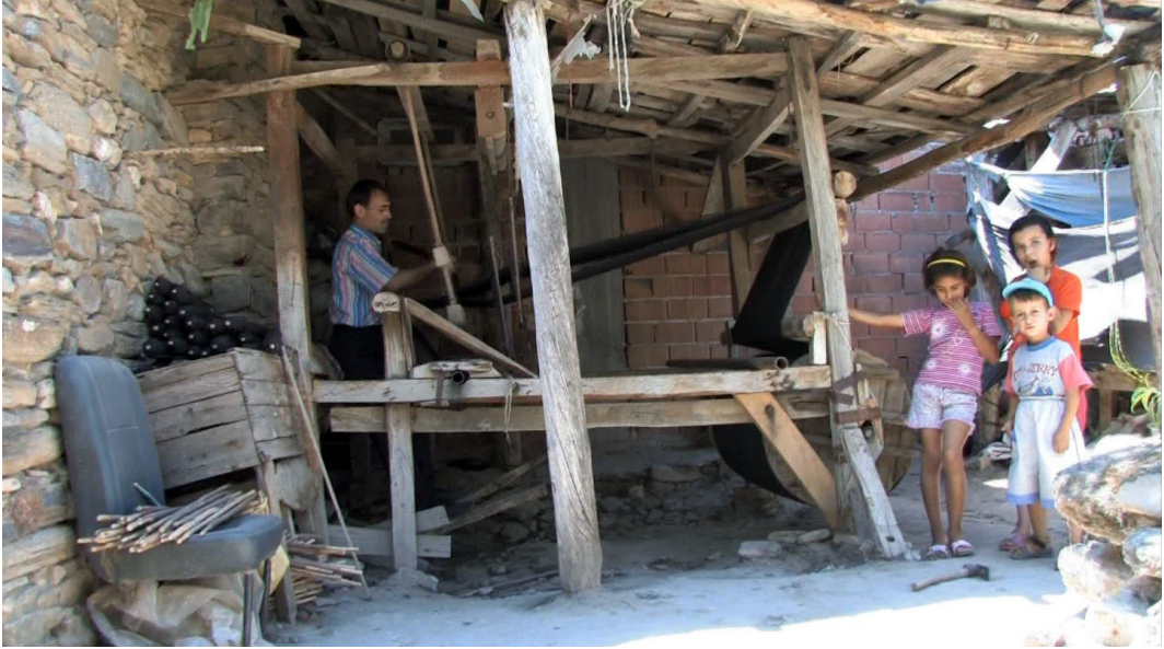
image 4.091: Treadle loom in Olukbaşı. On the left, on a car seat, empty bobbins made of wood are stored. Above, on the box, the bobbins are filled with yarn ready for use. The weaver sits or stands at the loom, handling the reed and the bobbin. Behind the reed, the two heddle harnesses can be seen. Below the loom, two treadles help navigating the harnesses. At the right, the warp is bent over two beams and rolled up over a cylinder. Here, panels up to a length of 27 metres can be done.
