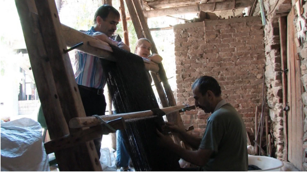
image 4.089: Total view at the three-bar loom with the third bar left out at the back.
