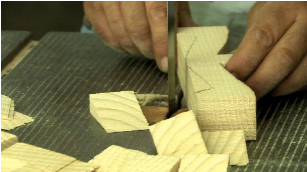
image 4.008: Similar to the ridge pieces, the stay-fasteners are cut out of the same type of pinewood.
