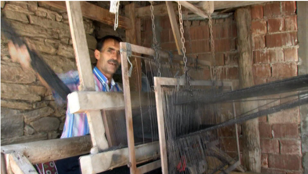
image 4.093: The heddle harnesses open and counter-open the shed.
