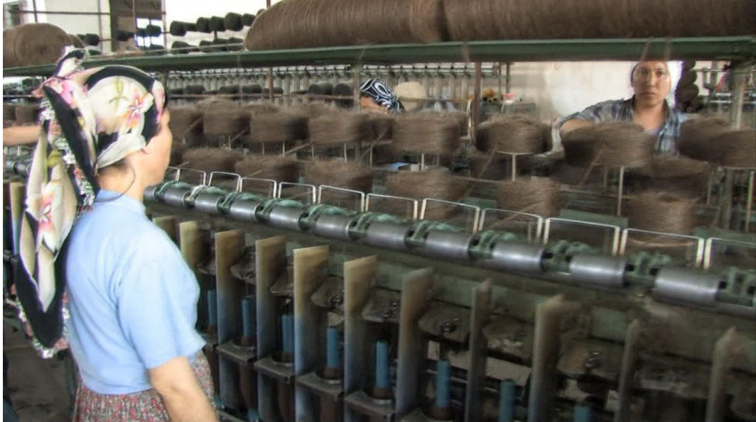
image 4.081: An extra machine spins the threads into a yarn and spools it to a bobbin that fits into the automatic weaving machines. Here, more personnel is needed for supervising and correcting the spinning. Also, the mounting and un-mounting of the bobbins must be done by hand.
