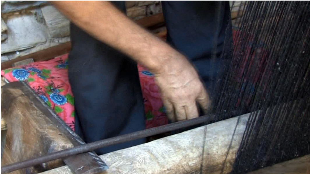
image 4.086: Looping the thread around the warping rod (made of metal in this case). The warping rod's purpose is only to ensure a continuous warping of the threads around the beams. When the weaving is started, it stays fixed to the end of the weft. As the warp is looped around the beams, it will be moved around them during the weaving process, carrying the warping rod upwards at the back of the loom.
