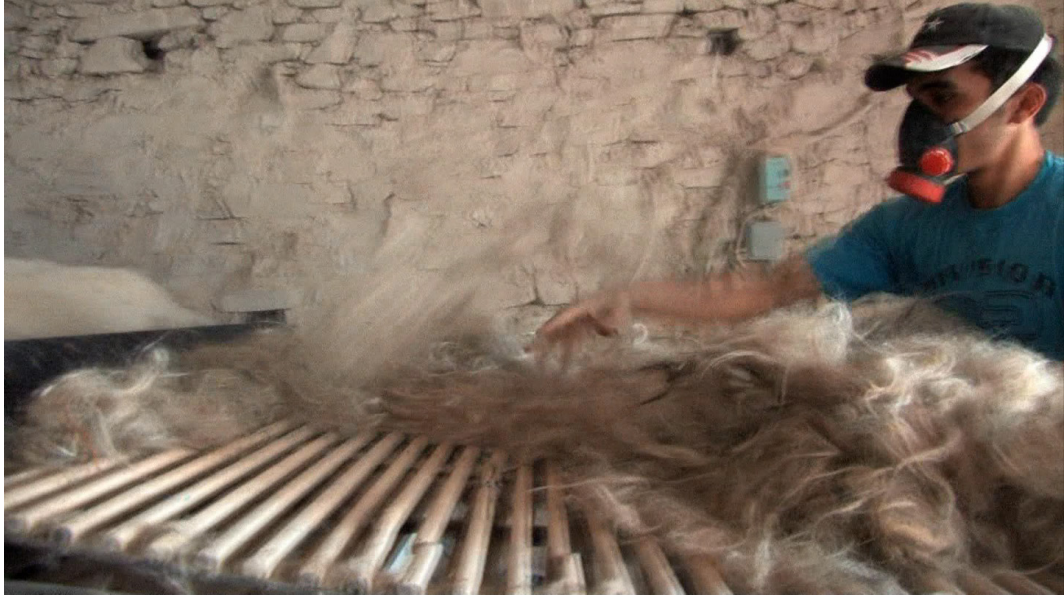
image 4.065: Wool being driven through a machine. The raw wool is laid out on the combing machine's pick-up tray and is then slowly taken up by rollers.
