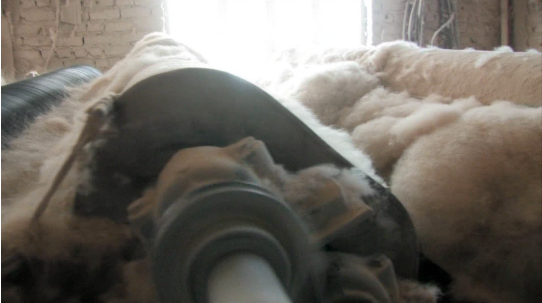
image 4.067: In the middle of the machine the downy hair is expelled, being manually collected by men periodically. This is analogue to the traditional way of collecting the downy left overs on a combing board which are carded on carding brushes in a second step.
