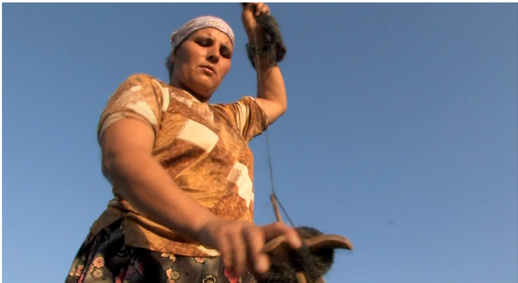
image 5.019: After three or four sequences of picking strands of roving, the spindle needs another twitch. The right hand runs down to the spindle, grabbing it at its arms and giving it another twist. Then, the hand runs back to its previous position keeping on picking the hair.
