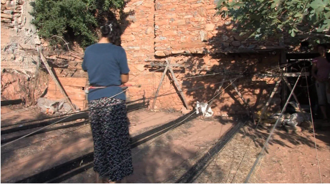
image 4.074: The spinner is connected to the cord with a belt bound to her waist. She moves continuously backwards and thus pulls the cord that drives the fly wheel. Likewise, unseen in this picture, she spins threads with her left and right hand each that are growing in length while she keeps moving. Therefore, she walks a certain path of length while activating the fly wheel. Readymade yarns are tucked to the ground at the left side of each spinning wheel. A yarn from the previous session is spun at the same moment when the spinner produces two new threads.
