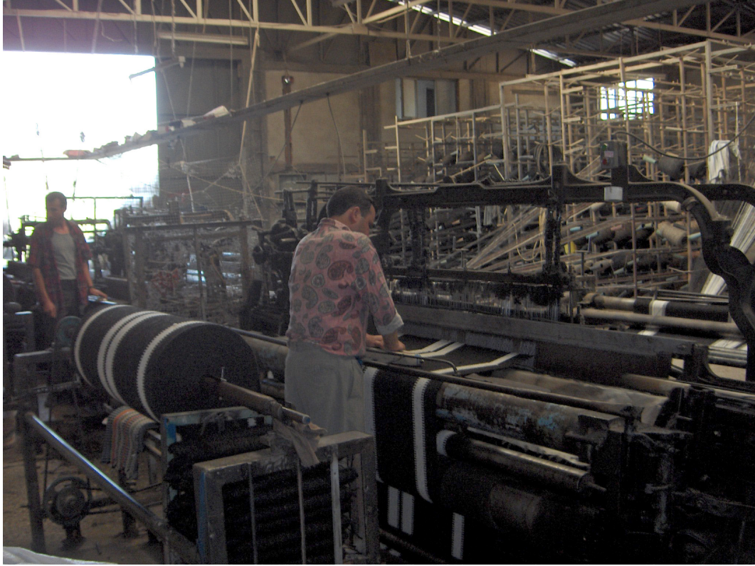
image 4.099: The weavers supervise the performance of the bobbin and occasionally need to correct little errors. The weft runs on rolls down below a platform to the backside of the weaver's working place where it is rolled up. Weaving machines produce panels at the length of up to 70 metres.
