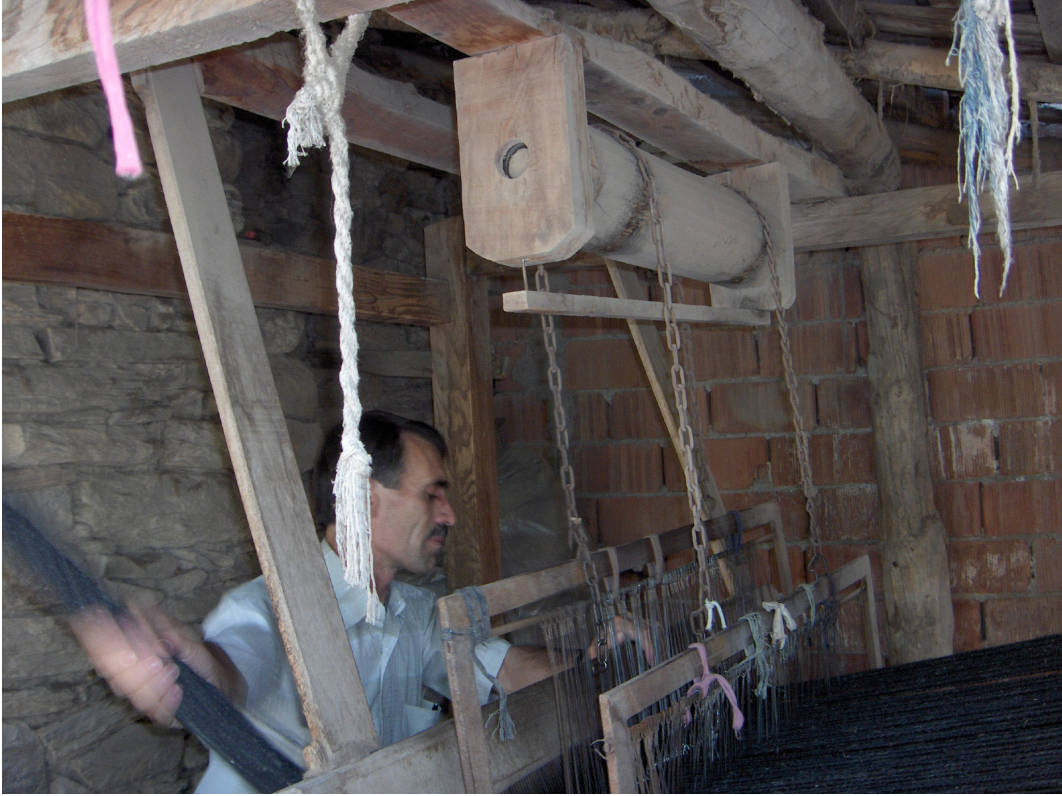
image 4.094: The harnesses are connected to chains running over rolls above. They are counter-balanced.
