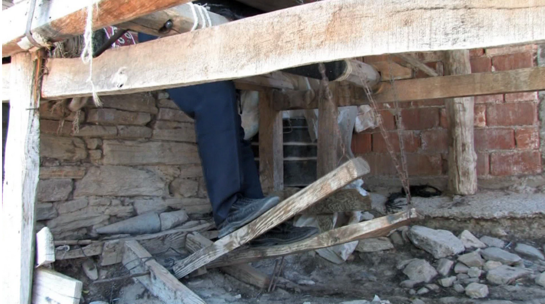
image 4.095: Below, the harnesses are connected to the treadles by which the up and down movement can be directed with the feet.
