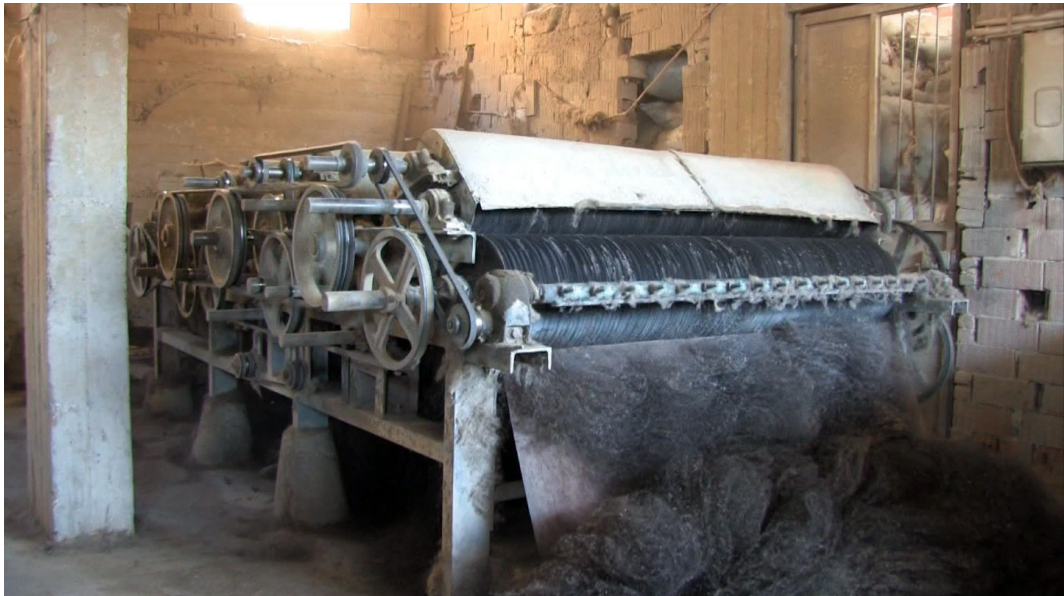
image 4.069: Overall view of a combing machine
