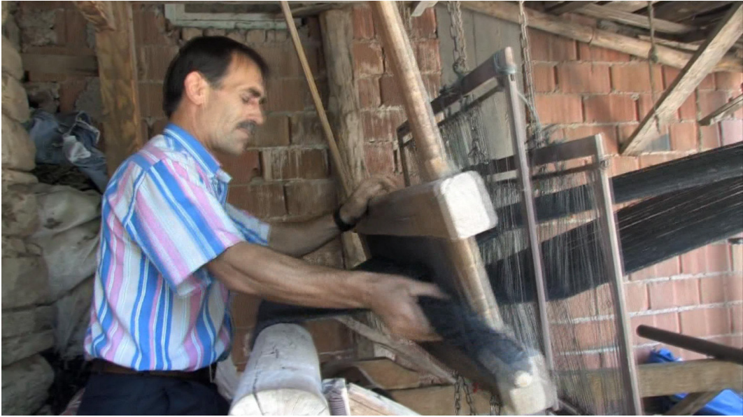
image 4.092: The bobbin is driven through the shed.
