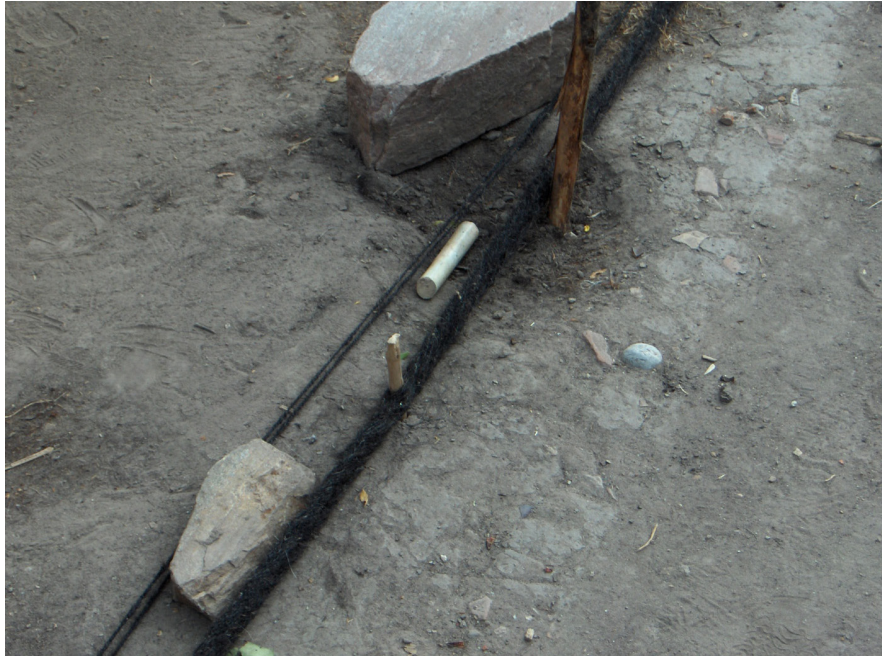
image 5.006: Rope made of goat's hair manufactured in the weavers' villages. The freshly twisted rope is fixed to the ground with a small stake.
