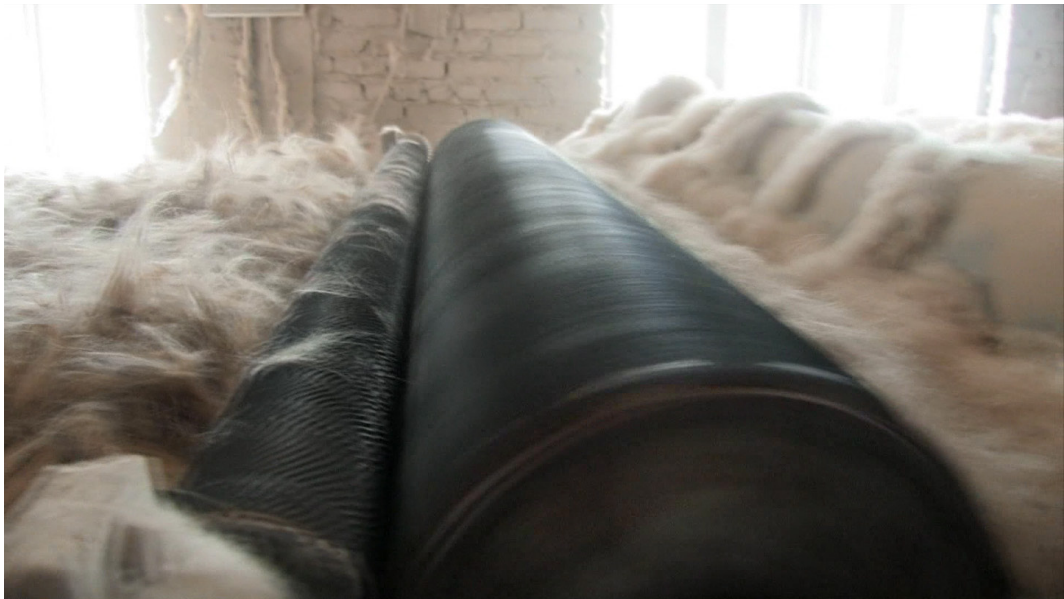
image 4.066: The wool is driven forward by several fine-toothed rollers on which rows of fine needles take the fibres apart by swift left and right movements along the axis. There, the wool is spread out over the whole width of the machine and cleaned from foreign particles. This process can be compared to the manual beating with a bow.
