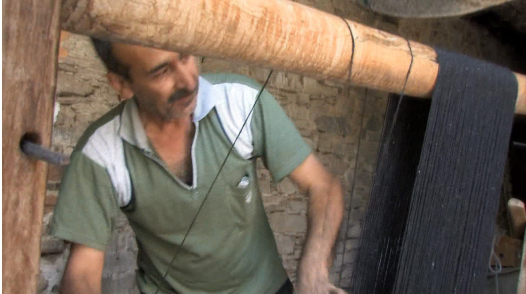
image 4.085: Running the warp thread over the upper beam.
