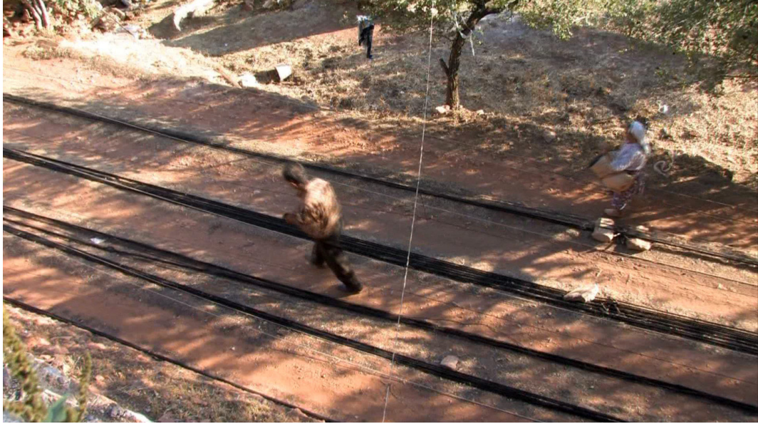
image 4.078: The spinning path is about of 30 metres length which defines the seamless length of the yarn. At the end of the path each yarn is cut and tucked down to the floor. After the spinning is done, the yarns are rolled up into a bundle being connected to each other with a single knot.
