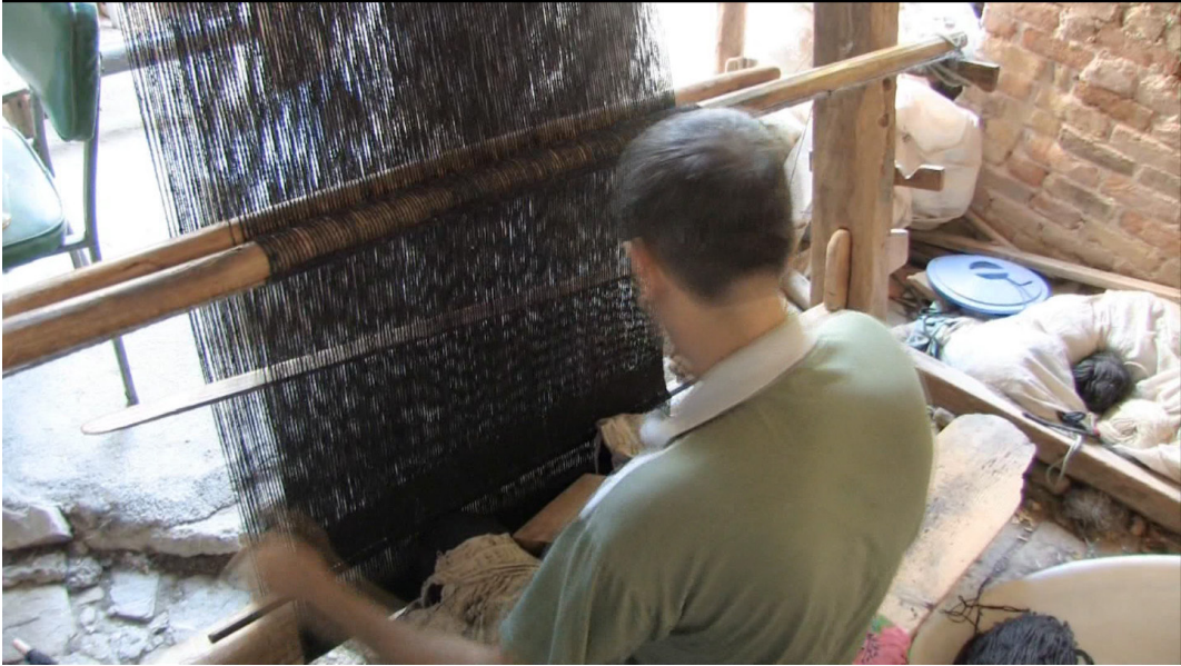
image 4.090: After the threading of the rod heddle is completed, the shed rod is stuck into the warp behind. Below, the sword beater can be seen. The weaver is about to drive a bobbin through the warp starting the weft. At the back of the lower beam the metal warping rod being fixed at the end of the weft can be seen. Now, during the weaving process, it will slowly move upwards with the weft at the back of the loom.
