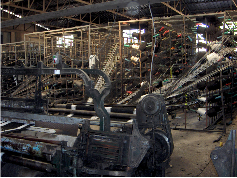
image 4.096: A mechanized loom in the factory hall of Olukbaşı. The spool rack feeds the warp for the loom. Here, a black tent cloth for Arab tents is produced. Contrary to the black goat hair threads, the white threads are herbal, made from cotton.
