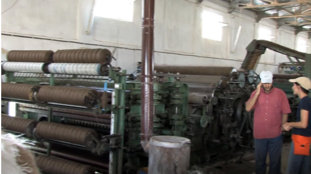
image 4.080: Automated machine combing and spinning the goat's hair into a thread in one process. At this stage, the counter-spinning to a yarn is not done yet.
