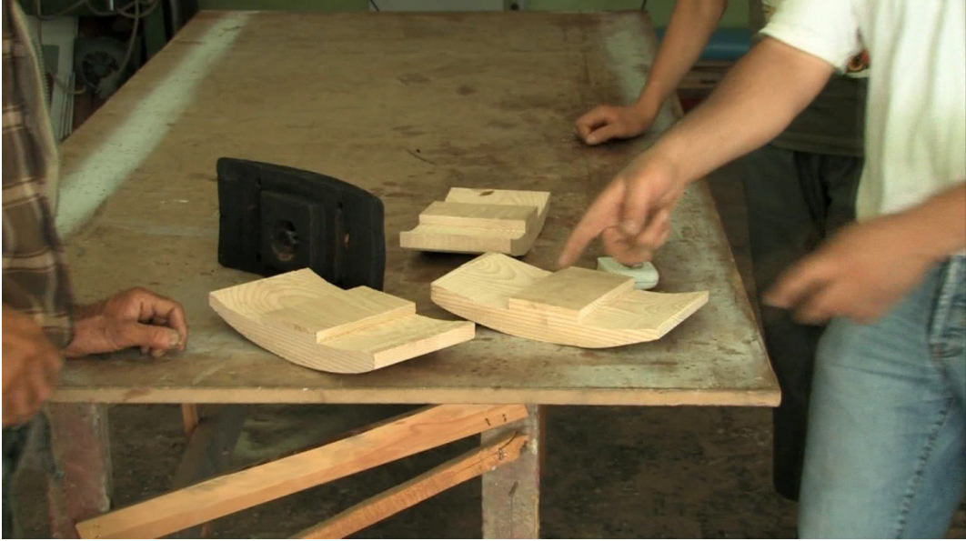
image 4.005: After a while we found a carpenter who would reconstruct the old ridge piece for us. The dark ridge piece derives from the old tent of the Şimşek family, being blackened from the fire fumes in the tent. It serves as a model for the new ones.
