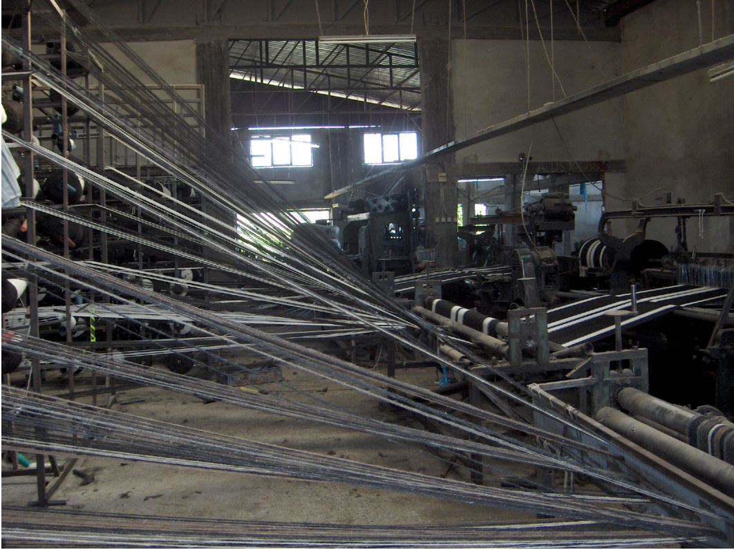
image 4.098: From left to right the yarn runs from the spool rack to the weaving machines forming the warp.
