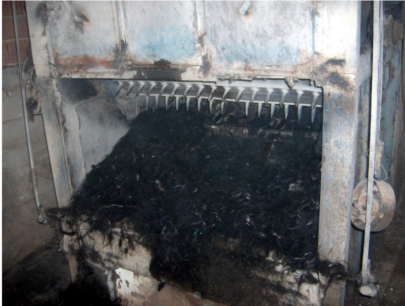
image 4.061: Drying and tumbling machine for raw hair and wool. Sometimes, alternatively, the drying is done by laying the wool out on the road being exposed to the warm sunlight.
