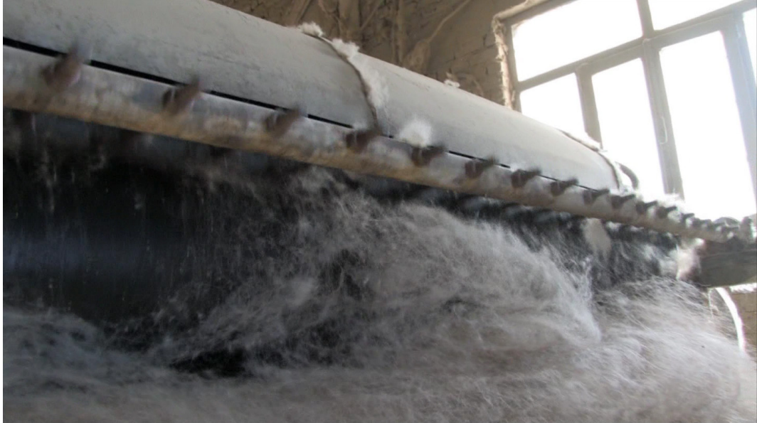
image 4.068: At the end of the machine a fleece of coarse kemp hair with parallel fabrics is laid out on the floor, being periodically collected by men and stored into sacks for spinning. This fleece may be compared to the brushes of straightened hair being obtained from the combing boards.
