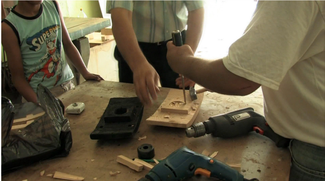
image 4.007: The trough of the ridge piece is carved out with a gouge. Then, with an electric drill, four holes -one for each corner- are drilled for fixation on the central panel later.
