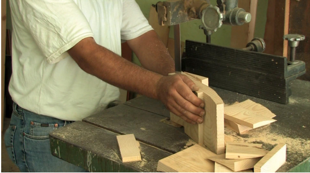
image 4.006: The ridge piece is cut out by the help of a belt saw.
