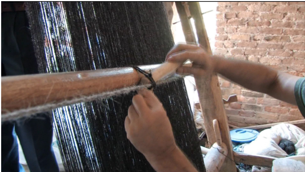
image 4.088: An extra thread is looped around the warp threads and the rod heddle.
