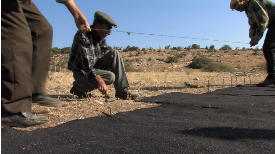
image 4.017: The pattern of the roof is laid out on the ground. The panels are pinned down to the ground with large nails made of steel. The fringe is evened out with a thread drawn across. In the middle of the image, Nasuh Şimşek can be seen, with 74 years of age he is the oldest tent builder within the group.
